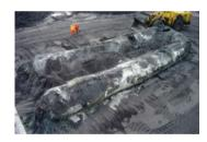
The company ESD-Sic b.v. in the Netherlands is one of the leading manufacturers of silicon carbide. During the production process, a mixture of pure quartz sand and petroleum coke is heated under a plastic tarpaulin to a temperature of approximately 2300° C by supplying electric energy with a rated voltage of 500 - 600 V, 50 Hz. Both source materials react to silicon carbide. The reactive power load of the process is 7000 - 8000 kVAr.
